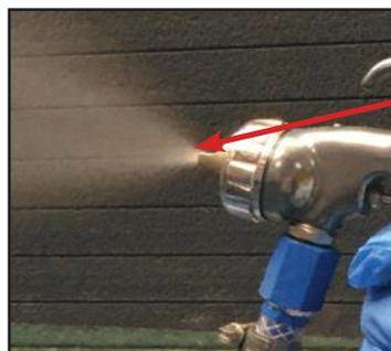
It is the use of air to atomise the adhesive which causes shear forces and breaks down the colloids.
