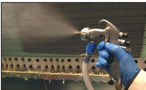
**Figure 5. 1-part water-based adhesive being sprayed**
